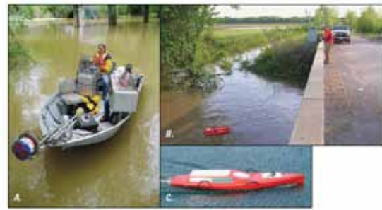
ADCPs are used on a variety of measurement platforms. (A) Manned boats (photograph by Paul Baker, USGS). (B) Tethered boats (photograph by Kevin Uberg, USGS). (C) Remotely controlled boat.
